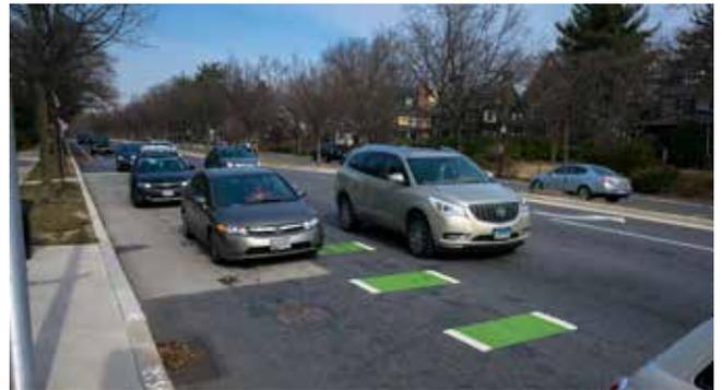
Bus stops near intersections tend to function as right-turn lanes for motorists, which places the bicyclists between and crossing with moving vehicles and creates conflict for buses entering and existing traffic.
