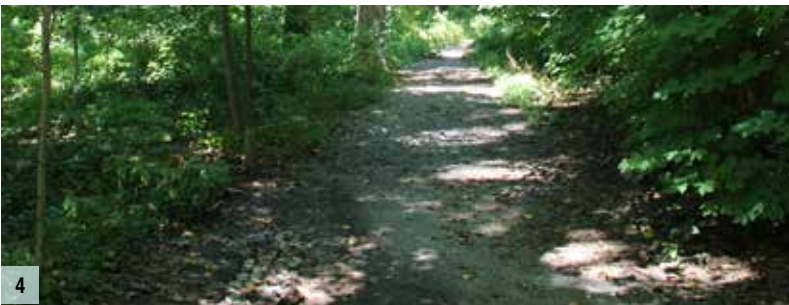
1: PAVEMENT (Asphalt) — Application: Formal park spaces, such as Linkwood Park. 2: MULCH PATH — Application: Gilman School to Wyndhurst Avenue. 3: BOARDWALK — Boardwalk over wet areas. Application: Oakdale Meadow and Linkwood Park. Pictured: Canaan Valley Resort State Park (Davis, WV). 4: PACKED EARTH/STONE DUST — Application: where currently used. 5: PAVEMENT MARKING — Application: Wyndhurst Station/Meadow Lane.
